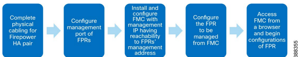
Figure 3-4: Workflow for Configuring Firepower
