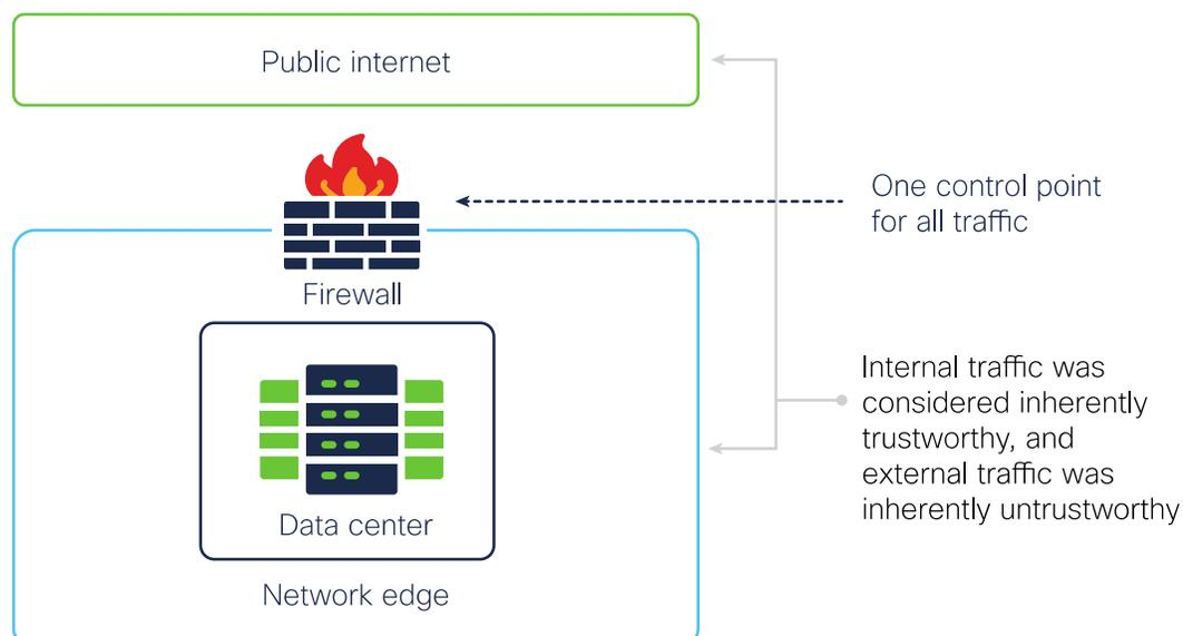
**Figure 1.** Traditional network firewall approach
